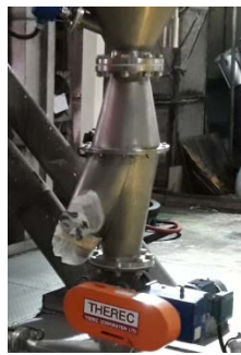
Air lock Rotary & Diverter Valve / Product Sampling Valve / Mitr Pukeaw Factory Sugar dust from vibrating screener. blow to packing machine
