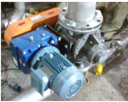
Air lock Rotary & Diverter Valve / Product Sampling Valve / Mitr Pukeaw Factory Sugar dust from vibrating screener. blow to packing machine
