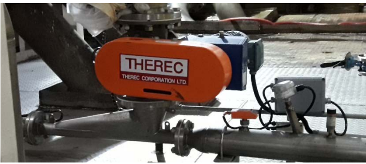
Air lock Rotary & Diverter Valve / Product Sampling Valve / Mitr Pukeaw Factory Sugar dust from vibrating screener. blow to packing machine
