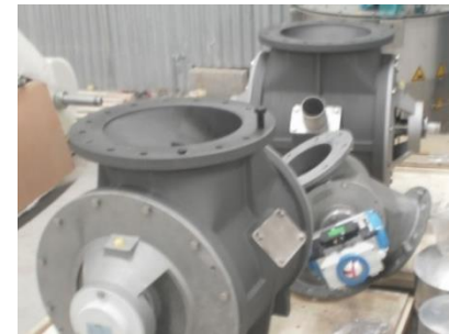
Non cutting Rotary valve (Granular Valve)
