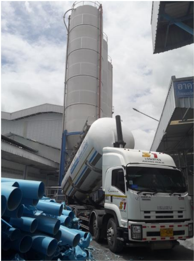
PVC & CaCo 3 Bulk Bag , Silo feeding system, 5 Tons / hr
