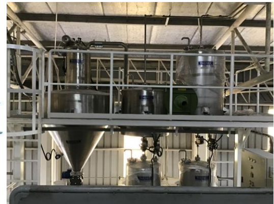
Stainless steel 304 PVC Resin Silo, Size 100 m 3
