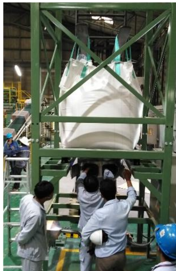
Big Bag Unloading Station Thai Plastic and Chemical (Public) Co.,Ltd. / TPC
