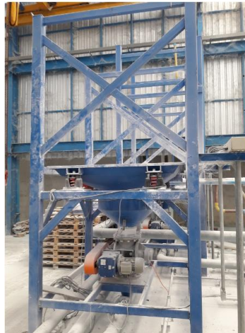
PVC & CaCo 3 Bulk Bag , Unloading station / Fork lift type
