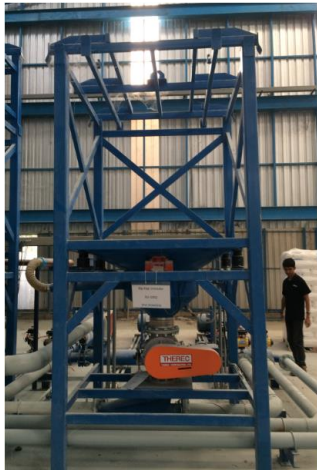
PVC & CaCo 3 Bulk Bag , Unloading station / Fork lift type
