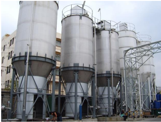
PVC Powder and CaCO 3 Powder Loading system
